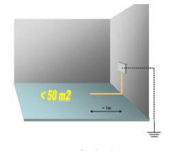
Picture 1 – Copper strip layout for rooms  $< 50 \text{ m}^2$
