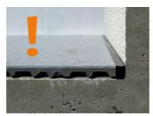
Wrong! A three-sided adhesion of PUR sealing compound inhibits free expansion and may lead to damages!
