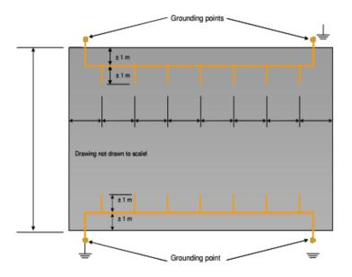
Picture 3 – Copper strip layout for rooms  $> 50 \text{ m}^2$ , alternative B
