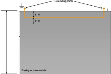
Picture 2 – Copper strip layout for rooms  $> 50 \text{ m}^2$ , alternative A
